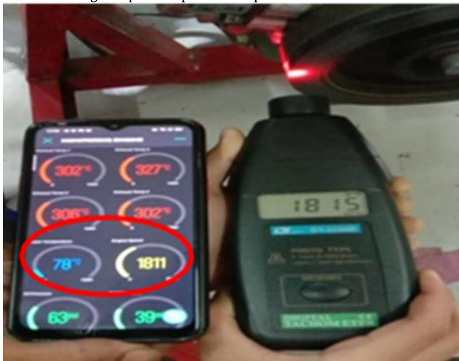
Gambar 10. Pengukuran engine speed
