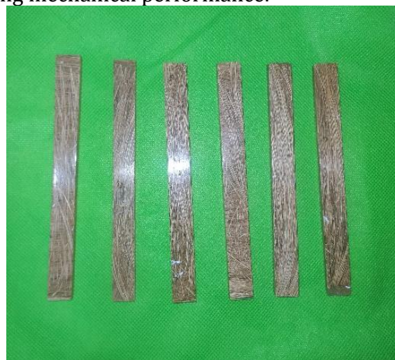
Figure 5. Coir Fiber Composite Specimen
