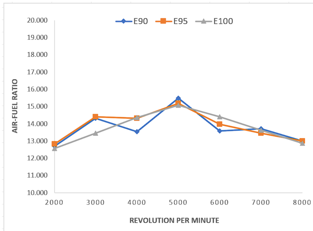
Figure 5. AFR trend of the 10-hole injector using E90, E95, and E100 fuel blends
