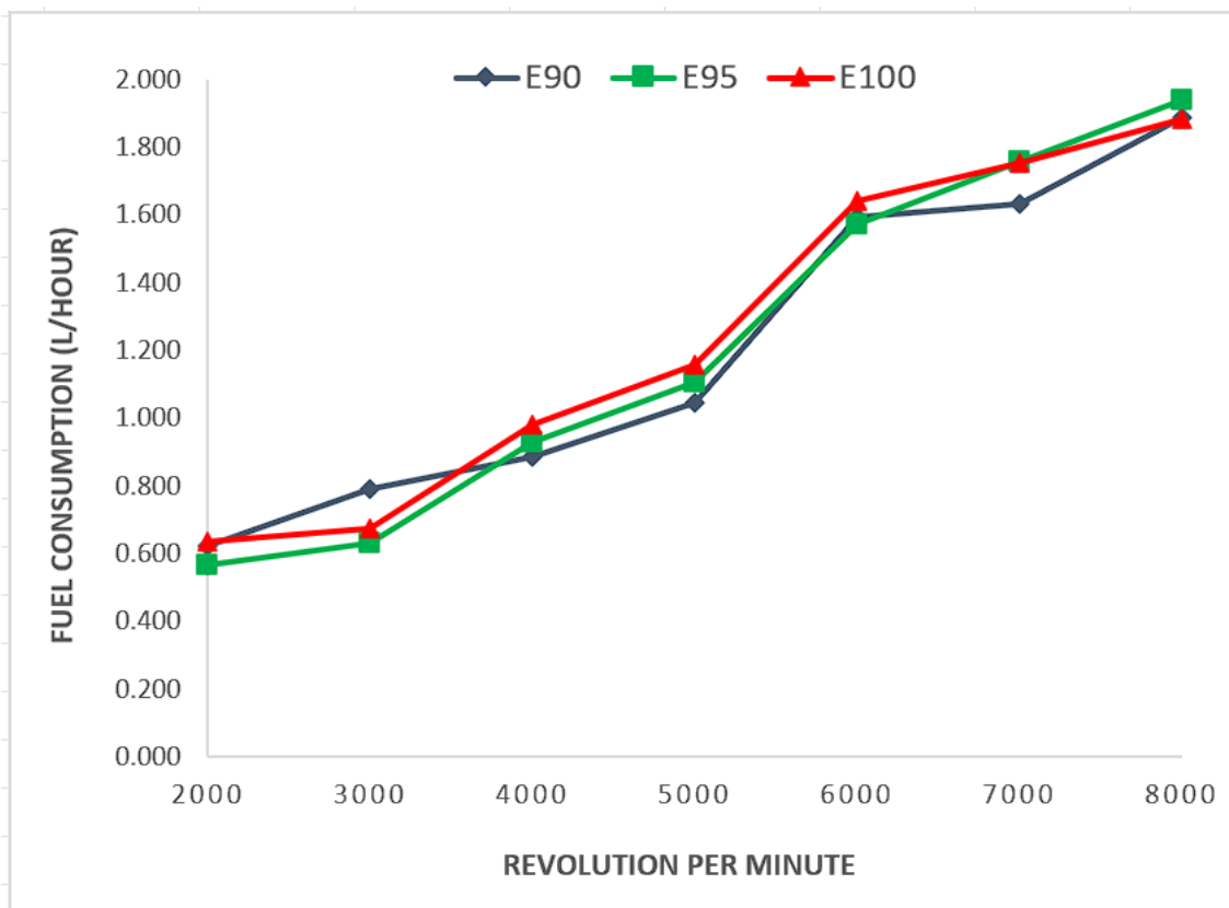
Figure 3. Fuel-consumption trend of the 10-hole injector using E90, E95, and E100 fuel blends
