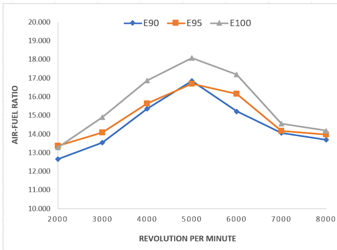
Figure 4. AFR trend of the 8-hole injector using E90, E95, and E100 fuel blends
