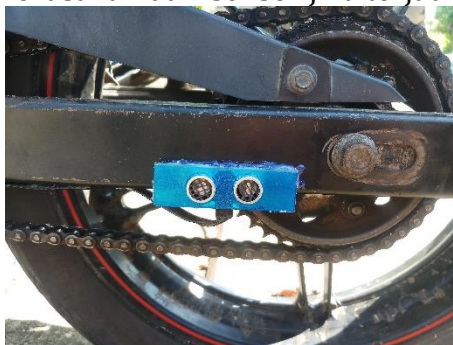
Gambar 4. Posisi Sensor Smart Alert
