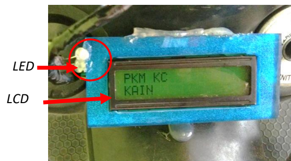
Gambar 6. Posisi LED dan LCD Smart Alert
