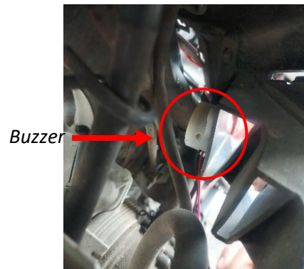
Gambar 5. Posisi Buzzer Smart Alert
